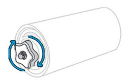
While holding the handle in place, twist the gear to adjust the grind.
